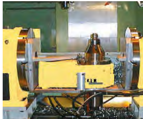
Machining of turbine wheel to use 2 units of CNC rotary tables, one for the swing axis of the HF motor and the other for the rotary axis of the work piece
