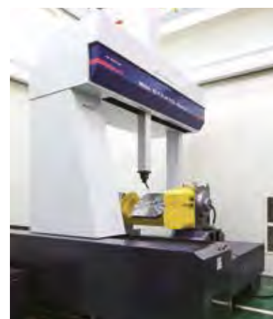
Accuracy measurement with large 3 Dimensional Measuring Machine
