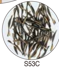
NC5-63 Material: S53C V=500m/min. f=0.25mm/tooth S=10000min -1 F=10000mm/min.
